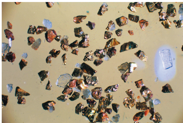
Figure 16. Example of the sulphide and matrix minerals in the sample I-F3. (40X magnification.)
