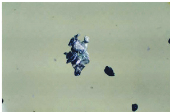
Figure 7. Amalgamated fine gold particle clusters, Saramacca River, Suriname (40X nominal magnification). These clusters were found in all tailings where mercury was used in the process. The high surface area in relation to volume of these clusters makes them more mobile and thus more easily lost.
